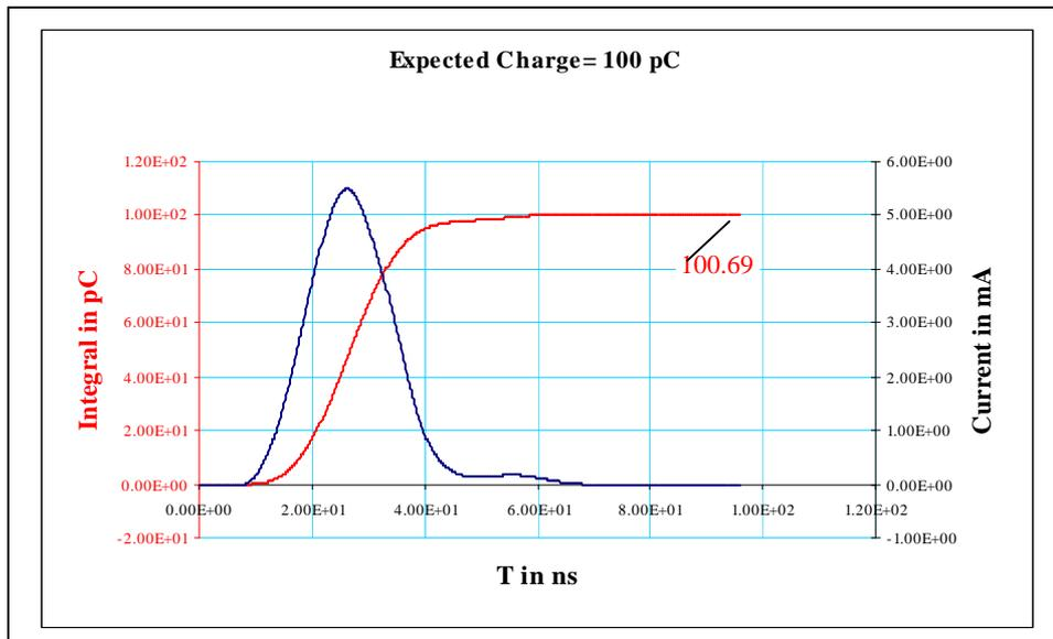
The above graph shows the rise of the Step generator (red) and the current impulse (blue) – the derivation of the voltage - of the Presco calibrator type PD-CLSB-CD00.
